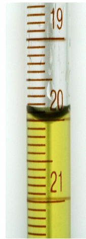
A meniscus as seen in a urette of colored water. '20.00 mL' is the correct depth measurement.
