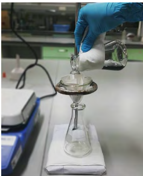
Figure 3.6.4: Filtration for the separation of solids from a hot solution. (CC BY-SA 4.0; Suman6395).
