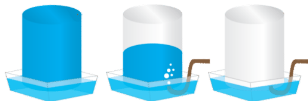
Figure 8.10.2: A gas produced in a chemical reaction can be collected by water displacement.
