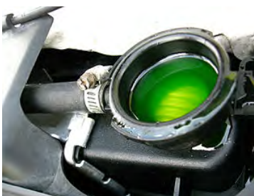
Fluorescent green-dyed antifreeze is visible in the radiator header tank when car radiator cap is removed. (CC BY-SA 2.0; EvelynGiggles)
