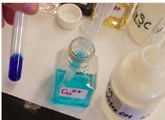
Figure 2.6.3: The Formation of Complex Ions. An aqueous solution of \text{CuSO}_4 consists of hydrated \text{Cu}^{2+} ions in the form of pale blue [\text{Cu}(\text{H}_2\text{O})_6]^{2+} (left). The addition of aqueous ammonia to the solution results in the formation of the intensely blue-violet [\text{Cu}(\text{NH}_3)_4(\text{H}_2\text{O})_2]^{2+} ions, usually written as [\text{Cu}(\text{NH}_3)_4]^{2+} ion (right) because ammonia, a stronger base than \text{H}_2\text{O} , replaces water molecules from the hydrated \text{Cu}^{2+} ion. For a more complete description, see www.youtube.com/watch?v=IQNcLH6OZK0 .
