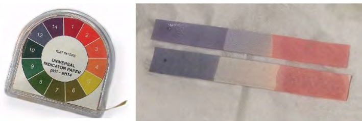
Figure 5.15.9: pH Paper. pH paper contains a set of indicators that change color at different pH values. The approximate pH of a solution can be determined by simply dipping a paper strip into the solution and comparing the color to the standards provided. (CC BY-SA-NC; Anonymous by request)
