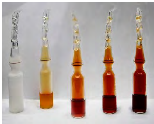
Figure 4.2.1: Dinitrogen tetroxide is a powerful oxidizer that reacts spontaneously upon contact with various forms of hydrazine, which makes the pair a popular propellant combination for rockets. Nitrogen dioxide at -196\text{ }^{\circ}\text{C} , 0\text{ }^{\circ}\text{C} , 23\text{ }^{\circ}\text{C} , 35\text{ }^{\circ}\text{C} , and 50\text{ }^{\circ}\text{C} . ( \text{NO}_2 ) converts to the colorless dinitrogen tetroxide ( \text{N}_2\text{O}_4 ) at low temperatures, and reverts to \text{NO}_2 at higher temperatures. (CC BY-SA 3.0; Eframgoldberg ).
