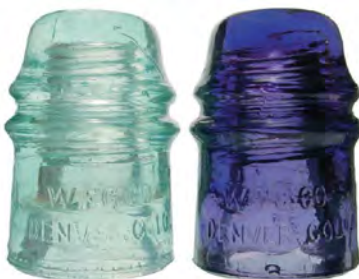
Figure 9.11.1: Radiation Damage. When high-energy particles emitted by radioactive decay interact with matter, they can break bonds or ionize molecules, resulting in changes in physical properties such as ductility or color. The glass electrical insulator on the left has not been exposed to radiation, but the insulator on the right has received intense radiation doses over a long period of time. Radiation damage changed the chemical structure of the glass, causing it to become bright blue. (CC BY-SA-NC; anonymous)
