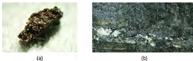
Figure 8.2.9: Naturally occurring free silver may be found as nuggets (a) or in veins (b). (credit a: modification of work by “Teravolt”/Wikimedia Commons; credit b: modification of work by James St. John)
