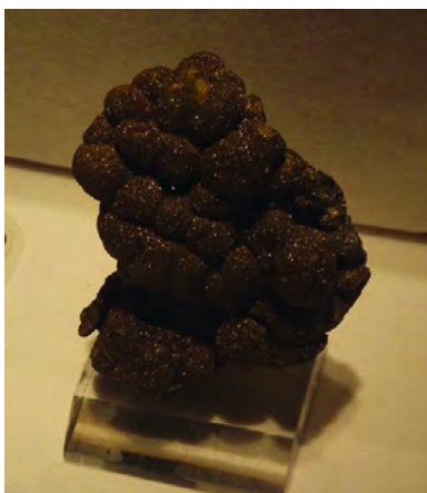
Figure 8.2.8: Blister copper is obtained during the conversion of copper-containing ore into pure copper. (credit: “Tortie tude”/Wikimedia Commons)
