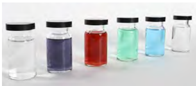
Figure 8.3.1: Metal ions that contain partially filled d subshell usually form colored complex ions; ions with empty d subshell ( d^0 ) or with filled d subshells ( d^{10} ) usually form colorless complexes. This figure shows, from left to right, solutions containing [M(H_2O)_6]^{3+} ions with M = Sc^{3+}(d^0) , Cr^{3+}(d^3) , Co^{2+}(d^7) , Ni^{2+}(d^8) , Cu^{2+}(d^9) , and Zn^{2+}(d^{10}) . (credit: Sahar Atwa)
