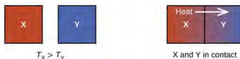
Figure 6.2.4: When two objects at different temperatures come in contact, heat spontaneously flows from the hotter to the colder object. Two separated blocks. One is labeled X and the other labeled Y. The diagram next to it shows the two blocks in contact with one another.
