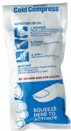
Figure 2.1.3: Commercial Cold Packs for Treating Injuries. These packs contain solid NH_4NO_3 and water in separate compartments. When the seal between the compartments is broken, the NH_4NO_3 dissolves in the water. Because \Delta H_{soln} for NH_4NO_3 is much greater than zero, heat is absorbed by the cold pack during the dissolution process, producing local temperatures less than 0^\circ C .
