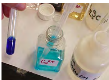
Figure 4.11.1: The Formation of Complex Ions. An aqueous solution of \text{CuSO}_4 consists of hydrated \text{Cu}^{2+} ions in the form of pale blue [\text{Cu}(\text{H}_2\text{O})_6]^{2+} (left). The addition of aqueous ammonia to the solution results in the formation of the intensely blue-violet [\text{Cu}(\text{NH}_3)_4(\text{H}_2\text{O})_2]^{2+} ions, usually written as [\text{Cu}(\text{NH}_3)_4]^{2+} ion (right) because ammonia, a stronger base than \text{H}_2\text{O} , replaces water molecules from the hydrated \text{Cu}^{2+} ion. For a more complete description, see www.youtube.com/watch?v=IQNcLH6OZK0 .
