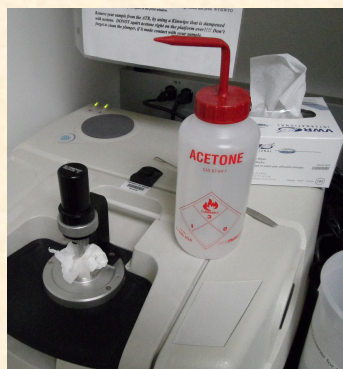
Clean ZnSe crystal and plunger with acetone damped Kimwipe.
