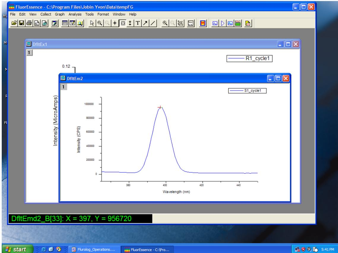
If the water-Raman peak is not at 397 nm, calibrate the emission monochromator.
