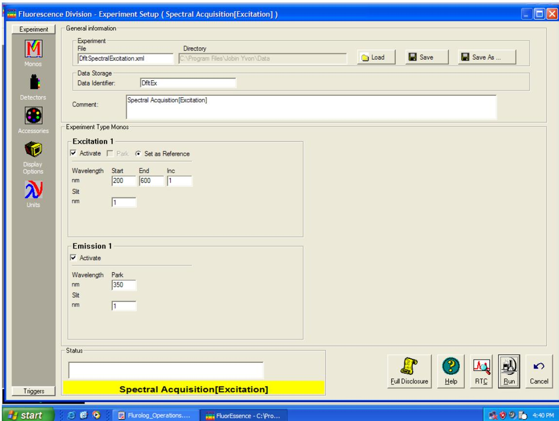
The Fluorolog will do an excitation scan on the xenon lamp.
