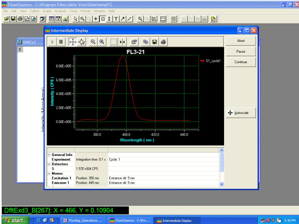
After the scan the screen will display the spectrum and you can use the data reader to inspect the wavelength max.
