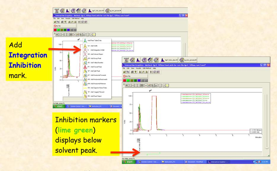
24. Stretch inhibition markers so all peaks with retention times greater than the solvent is ignored in the analysis.
