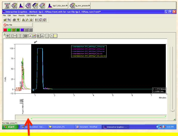
Click on right handle of inhibition marker and stretch to the end of time line so rest of signals are inhibited for integration in the analysis.
