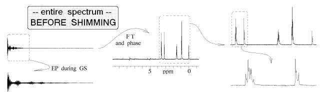
The main advantage of monitoring the FID of a *single, sharp* NMR line rather than the FID of an entire spectrum is that the envelope should be a simple, decaying exponential. You can be sure that any deviations from this ideal shape must arise from the magnetic field gradients which you are trying to cancel with the shims.
