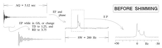
ALTERNATELY ADJUST Z, Z2, Z, Z2, ETC. YOU WANT TO MAXIMIZE THE AMPLITUDE OF THE LOCK SIGNAL, as indicated by its height on the graphics display screen. Reduce the lock receiver gain as needed to keep the lock-signal display a few cm down from the top of the screen. If the FID looks very bad, then the shims are very far out of adjustment and the lock-signal response to the shims might "feel" vague.
