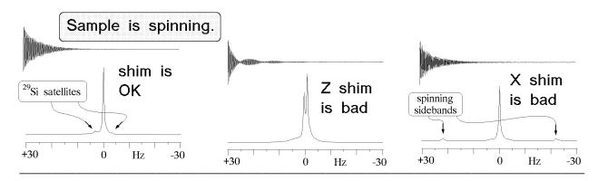
A bad FIRST-ORDER gradient is easiest to see in the FID. Beats in a FID mean small line splittings in the spectrum, and the signal from a single NMR line should not have any! Multiplet splittings will also produce beats in a FID, but these beats will not be affected by shim adjustments. Nulls arising from a bad Z shim, however, can be made to move to the right and disappear off the right end of the FID as you adjust the shim control.
