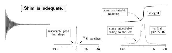
IN MOST CASES, IT IS FAR MORE IMPORTANT TO HAVE A GOOD LINE SHAPE THAN TO HAVE THE UPPER PART OF THE LINE BE AS NARROW AS POSSIBLE. The advantages of good line shape are better sensitivity (in most cases), the ability to accurately compare integrals of lines which are closer together, and the ability to apply resolution-enhancement techniques.
