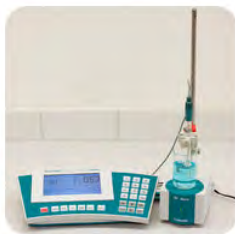
Figure 11.14.1: A pH meter is a laboratory device that provides quick, accurate measurements of the pH of solutions. (CC BY-NC; CK-12)
