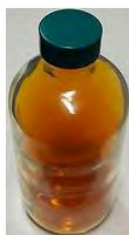
Figure 6.8.2: Nitrogen dioxide ( \text{NO}_2 ) is a reddish-brown toxic gas that is a prominent air pollutant produced by internal combustion engines.
