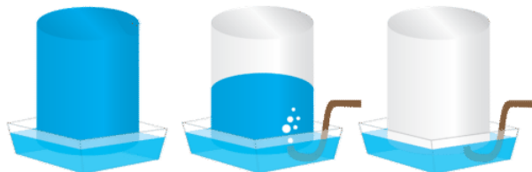
Figure 8.10.2: A gas produced in a chemical reaction can be collected by water displacement.
