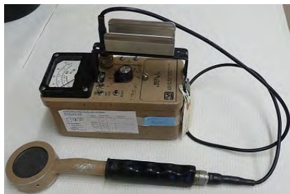
Figure 5.4.1: Detecting Radioactivity. A Geiger counter is a common instrument used to detect radioactivity.
